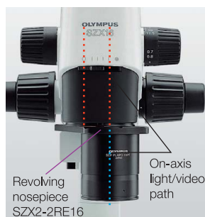
The nosepiece enables vertical observation.
